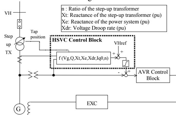
Figure 2-1. Configuration of HSVC control system
