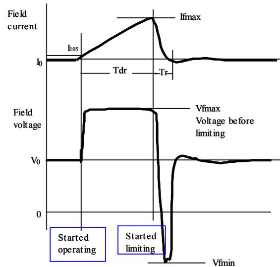
Figure 3-3. Behavior of field voltage and current
