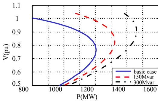
(a) P-V curve (static var compensator)
