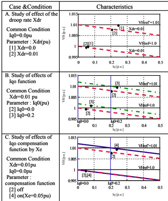
Initial Condition :  $P_1 = 0.9 \text{ p.u.}$ ,  $Q_1 = 0.04 \text{ p.u.}$ ,  $V_{Href} = 1 \text{ p.u.}$
