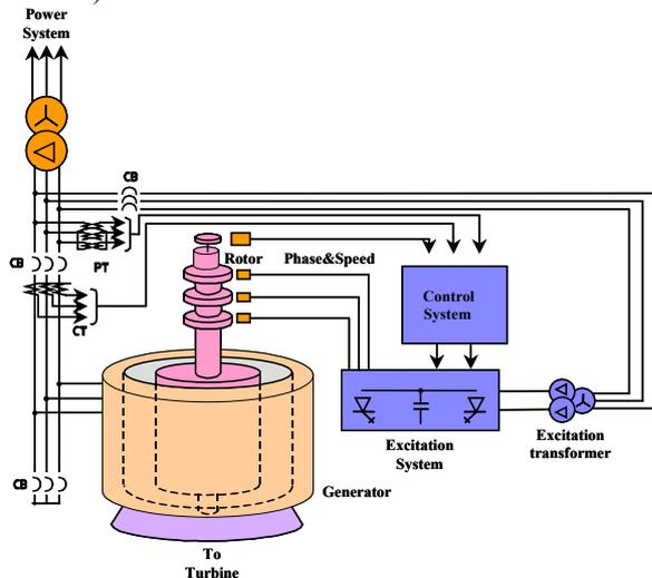
Figure 4-1. Concept of an adjustable speed machine
