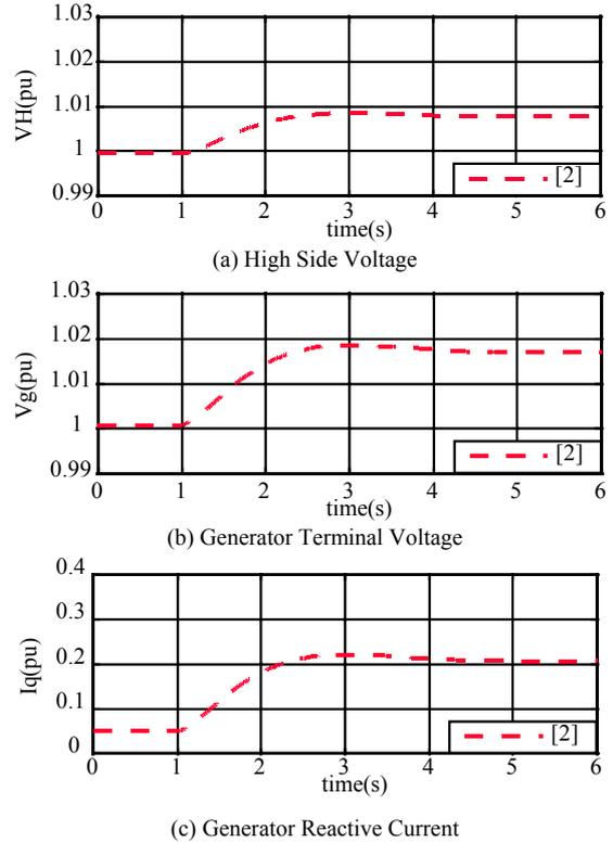
Figure 2-6. Response characteristics of the HSVC shown in Case C, in the points labeled [2] in Figure 2-5
