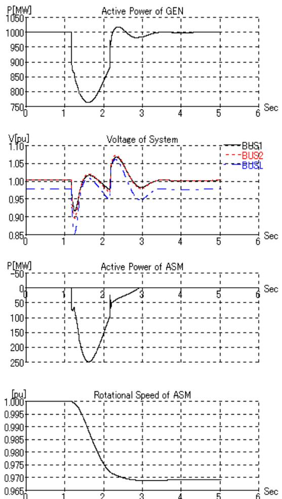
Figure 4-5. System responses after 1 line tripped (with voltage dip detecting function)
