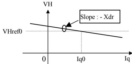
Figure 2-4. Characteristics of reactive current compensation function
