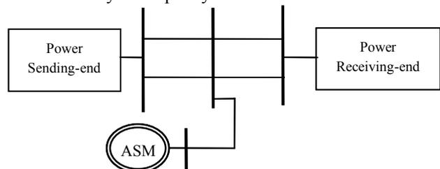
Figure 4-2. Illustration of an ASM condenser application
