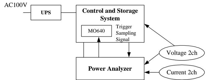
a) The Configuration of Measurement System
