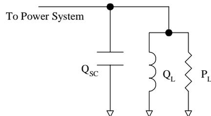
Figure 1. Illustration of Load in Power System on an Example Feeder
