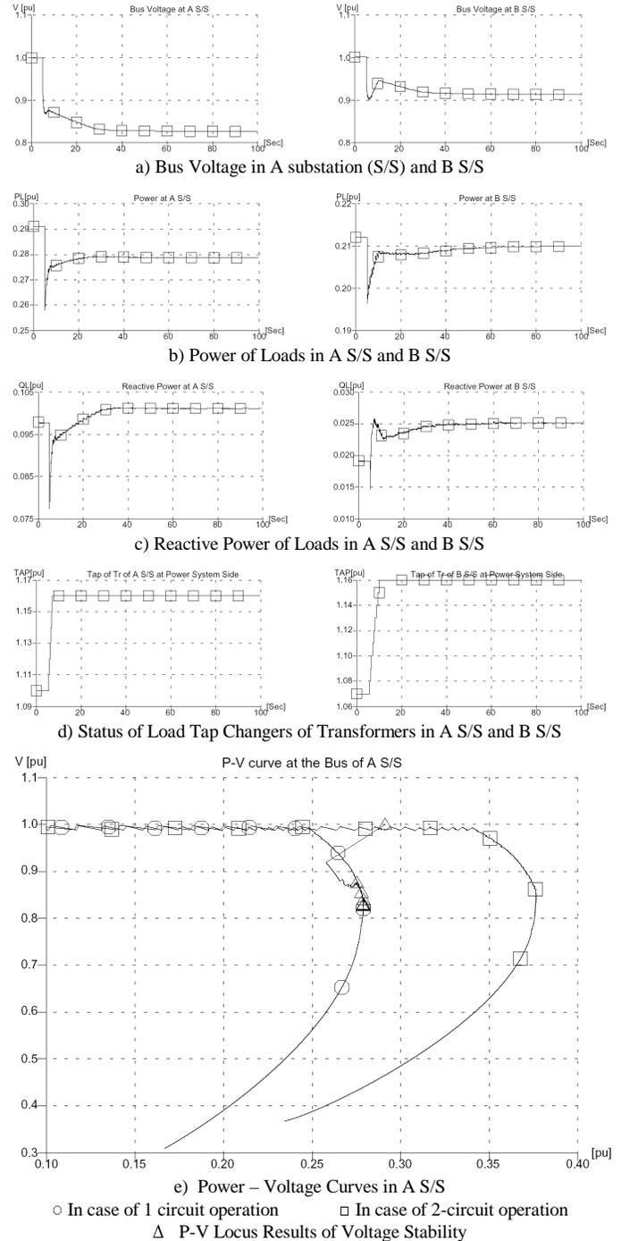
Figure 13. An Example of Results for Voltage Stability Analysis Using the Suggested Load Model
