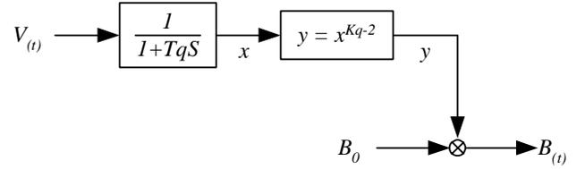
b) Reactive Power (Q) Model of Load
