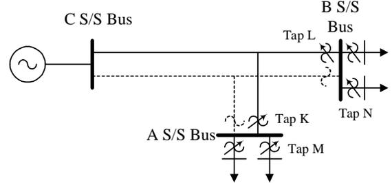
Figure 11. A Sample System for Voltage Stability Analysis
