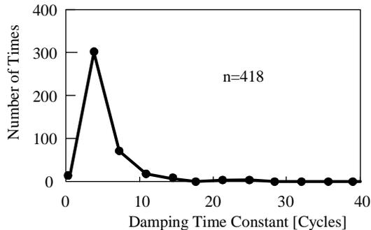
Figure 5. Distribution of Time Constants Calculated for 418 Cases of Measured Faults Over a Time Period of 10 years
