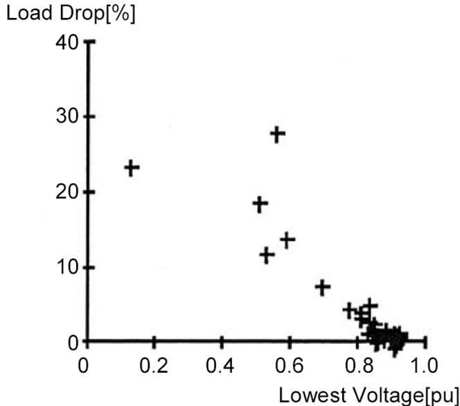
Figure 4. Measured Data of Load Drop by Faults
