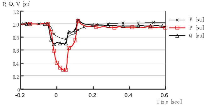
Figure 7. Measured Results of P, Q, and V in a Substation
