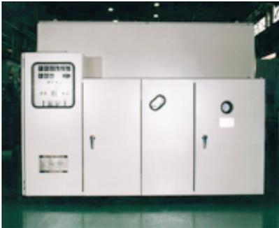
*Mitsubishi Electric* offers SF6 gas insulated Generator Main Circuit Breakers (GMCB) for applications in combustion turbine, combined cycle and other types of power plants. A GMCB is used to electrically disconnect a generator from the associated power transmission system, and sometimes is used to connect the generator to the static thyristor or other starting system in a combustion turbine plant. A GMCB is also common in a hydroelectric pumped-storage power plant.
